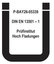
Fasatan<sup>®</sup> TFS is tested quality in compliance with DIN EN 13501, part 1 and corresponds to the building material class normally inflammable (DIN EN 13501 – class E), when our construction sealing foils Fasatan<sup>®</sup>, Fasatyl<sup>®</sup> and Fasatan<sup>®</sup> eco are adhered to metals, wood, or solid mineral subsurfaces with Fasatan<sup>®</sup> TFS.
