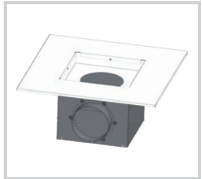
Return air connection box
