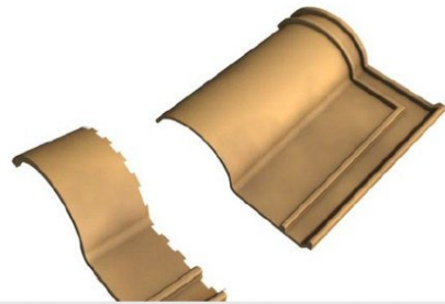
Tiles cutting for top flashing
